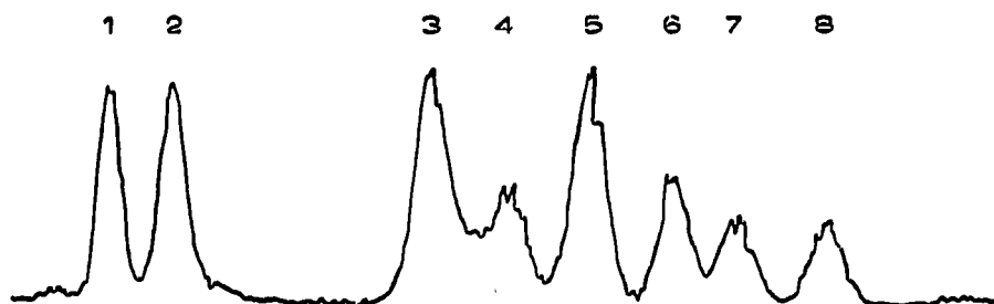
Fig. 2. Densitometric scan of TLC plate. Typical separation of the eight estrogen spots on the thin layer chromatogram with their corresponding recorded and integrated density curves. The peaks are numbered to correspond to Table I.
